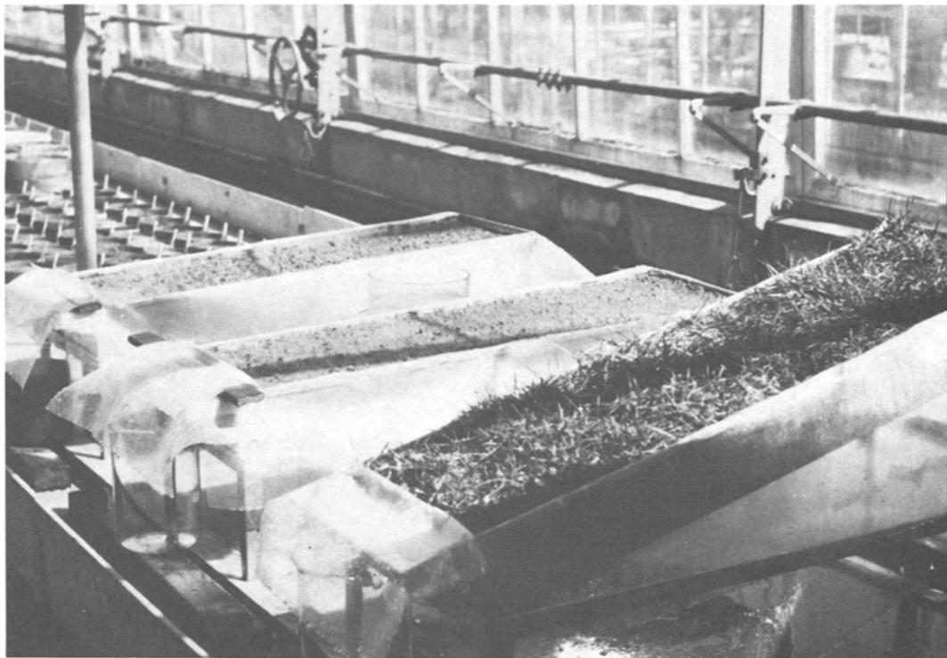
Figure 1 - Simulated field soil and turf plots used in greenhouse run-off and leaching studies
